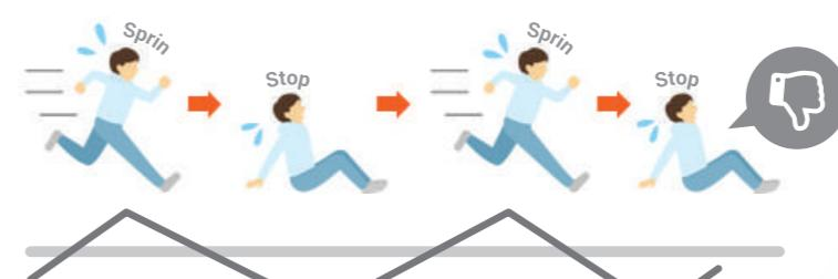
The non-inverter system continually starts and stops to maintain at the preset temperature. The repeated start-and-stop operation requires excess energy to restart the motor, resulting in energy wastage.
